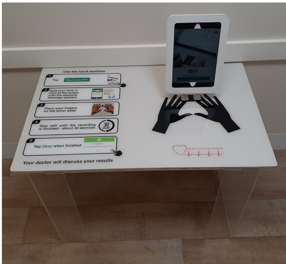
Fig. 1. Atrial fibrillation self-screening station.
